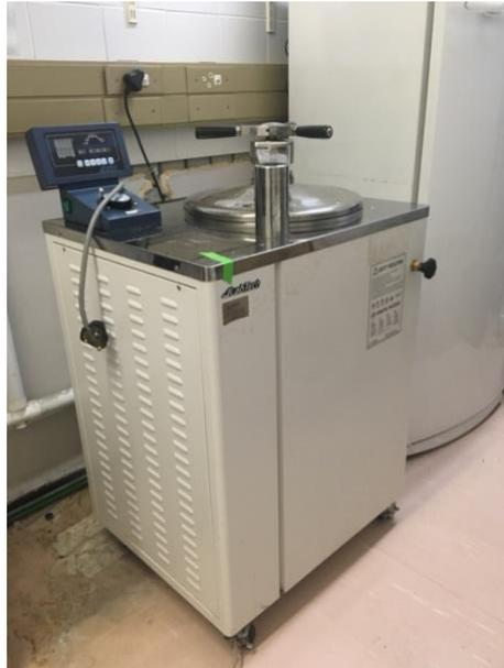
Figure 3.1: Autoclave used in the study for glassware and nutrient media sterilisation
