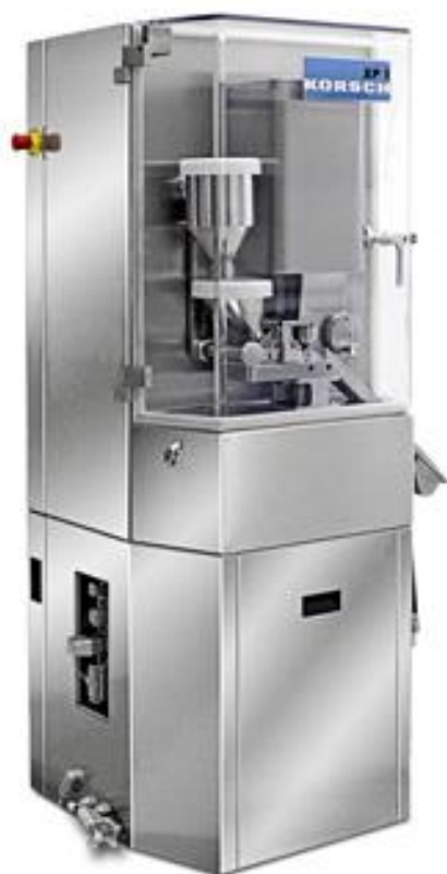
Figure 5: The Korsch Xp1 single punch tablet press used in this study (Korcsch, 2017)
