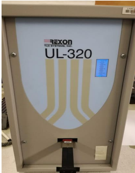
Figure 3.8: A REXON UL –320 TLD reader used for reading TLDs at the research site (Images acquired by the researcher for this research purposes)
