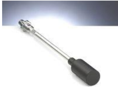
Figure 3.1: A PTW - Freiburg 30 cm 3 cylindrical ionization chamber.
