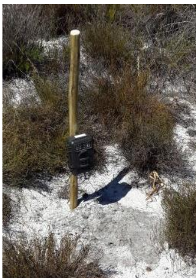
Figure 3.1: Remote sensing camera trap setup example - camera trap is secured on a wooden pole at 30 cm above ground level.
