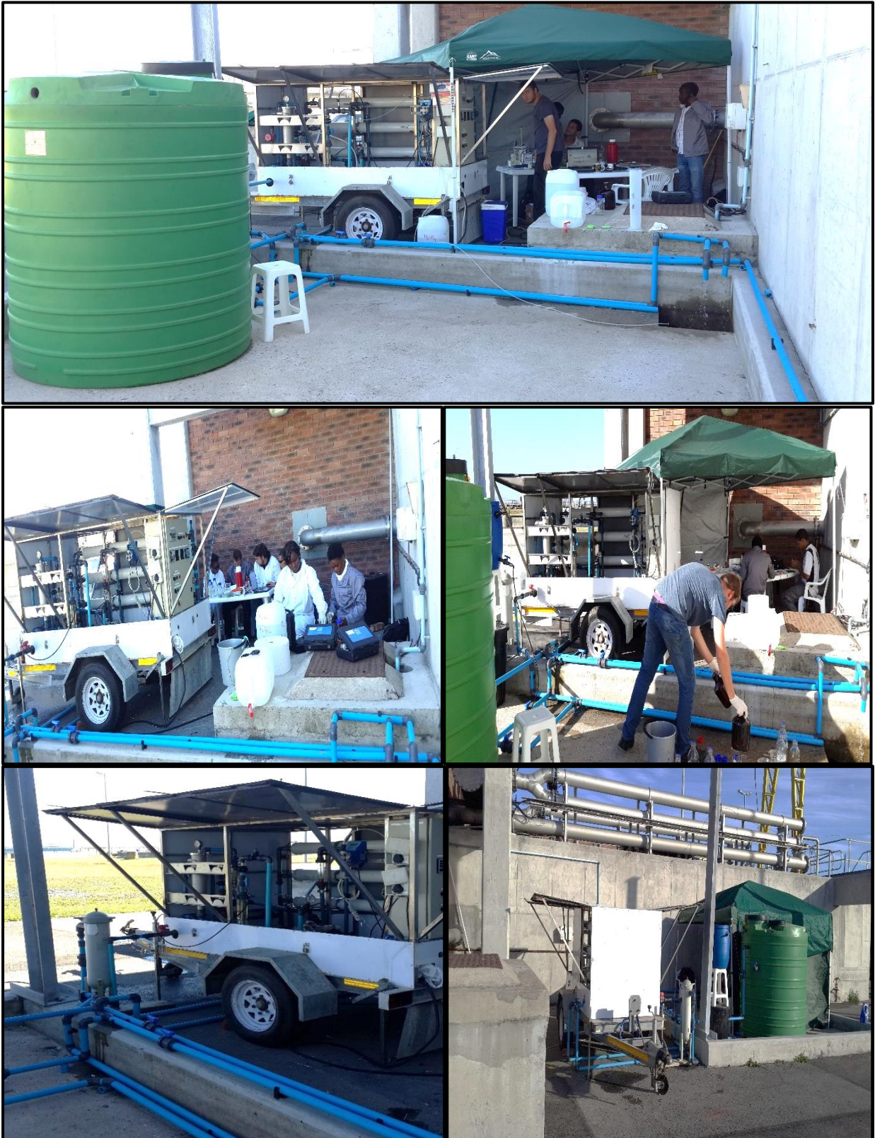
Photograph 3.3: (from top to bottom) Pilot plant on wheels linked directly to the MBR effluent.
