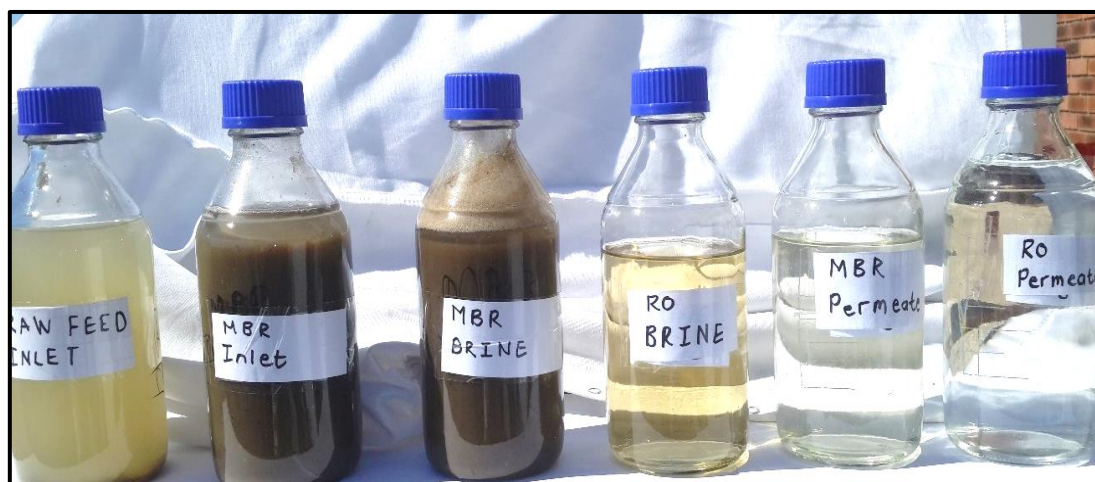
Photograph 5. 1: Samples showing the turbidity at different steps of the MBR/RO process
