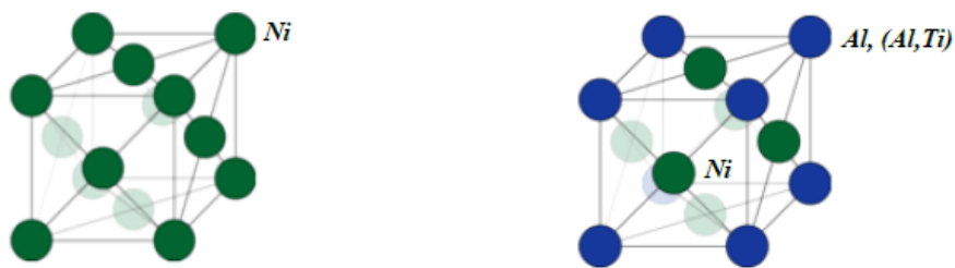
Figure 2.27: Two main crystal structures in a nickel-based super alloy FCC \gamma (left) and \gamma' (right) (Markusson, 2017)
