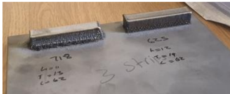
Figure 2.9: 3D additive manufacturing Inconel 625 and 718 sample specimens
