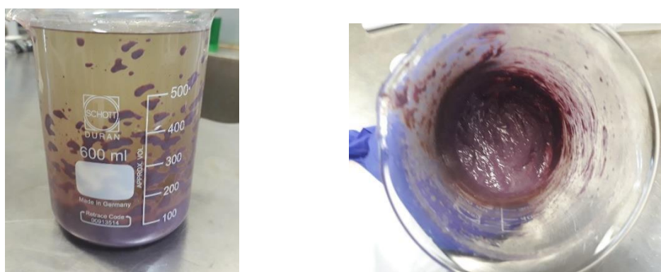
Figure 5-1: 100% octanol precursor after pH correction
