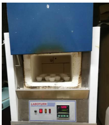
Figure 3-2: LABOFURN furnace used for calcination
