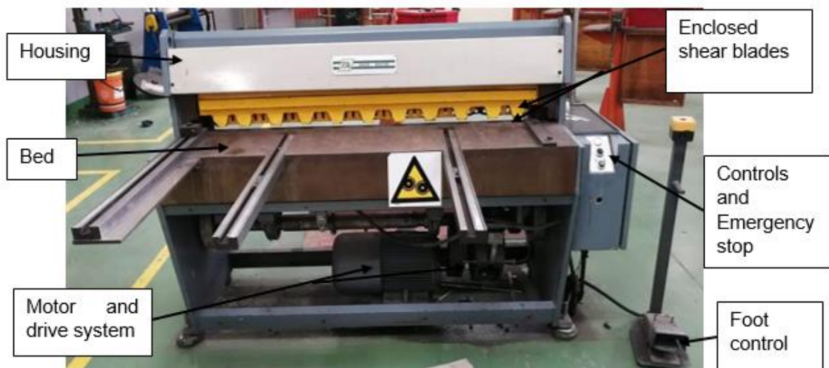
Figure 3.1: Shows the picture of a Guillotine Machine
