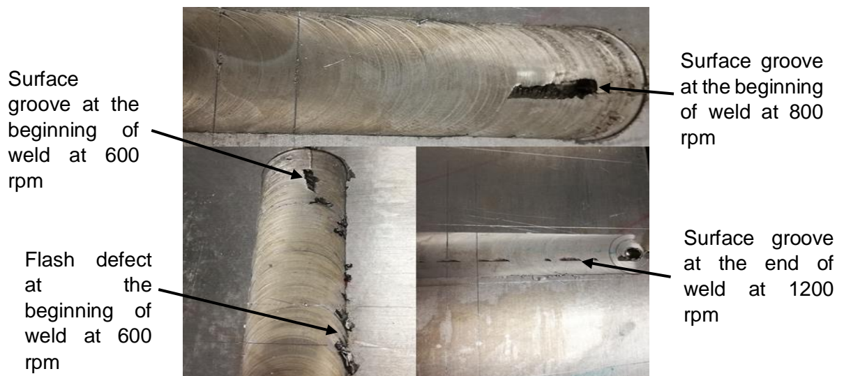
Figure 4.30: Shows the lack of fill on 600, 800 and 1200 rpm welds
