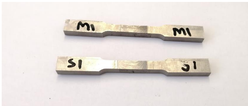
Figure 3.12: Cut out tensile specimens of 600 rpm from start and middle
