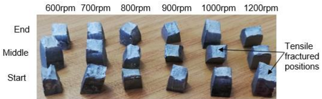
Figure 3.21: Cut off fractured tensile specimens
