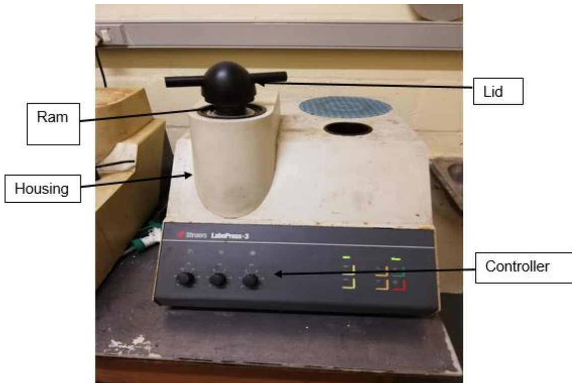
Figure 3.7: The Struers LaboPress-3 mounting machine with specimen after mounting
