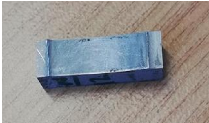
Figure 3.14: Shows cut-out microstructure specimen welded at 1200 rpm.
