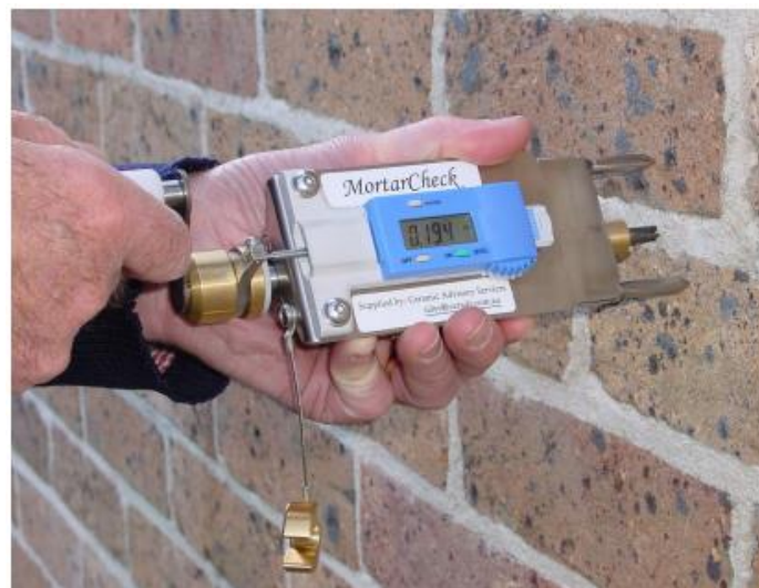
Figure 2.14 Mortar Scratch test (Lawrence et al. , 2004)
