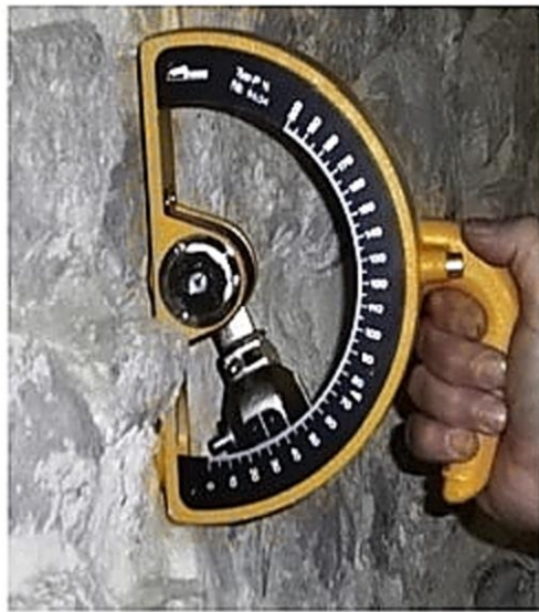
Figure 2.13 Pendulum Schmidt hammer (Schueremans et al. , 2011)
