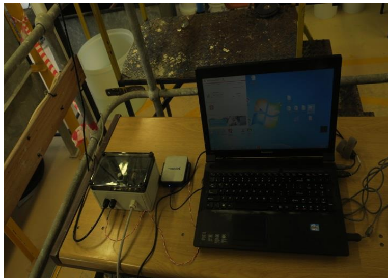
Figure 3.12 Connection of the data acquisition system to the computer
