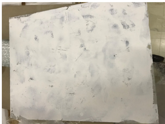
Figure 4-2: Glass coated with \text{TiO}_2 paste
