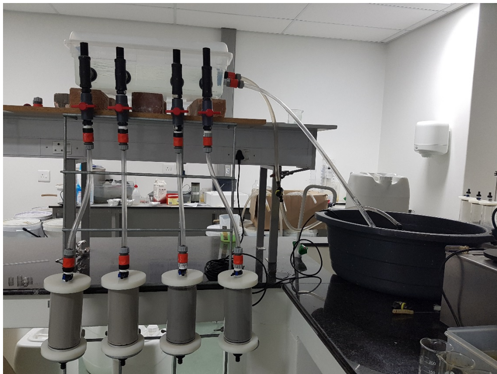
Figure 3. 7: Hydraulic column leaching system
