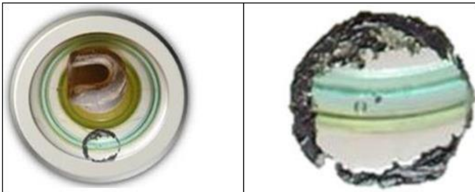
Figure 5-12: More than 70% of the contaminated area is now visibly clean after 135 seconds.
