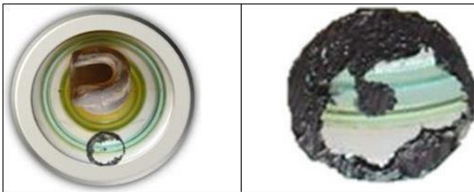
Figure 5-10: The contaminated area after 45 seconds of cleaning.
