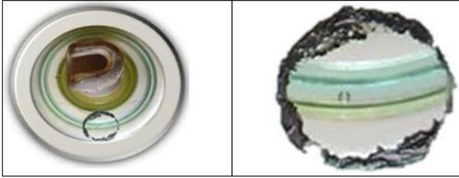
Figure 5-13: The grease under the transducer face is removed, after 180 seconds.
