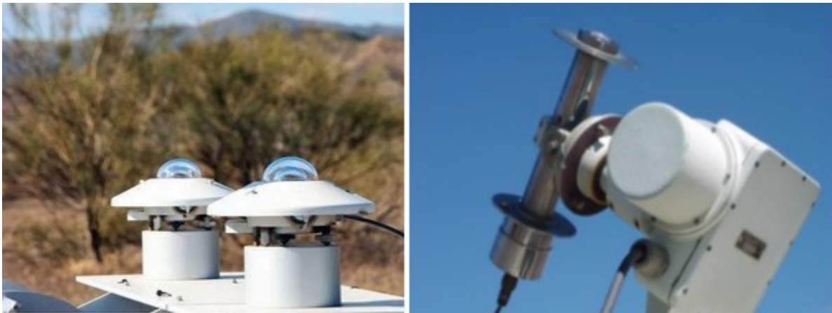
Figure 3-2: Pyranometer (left), Pyrhelimeter (right)
