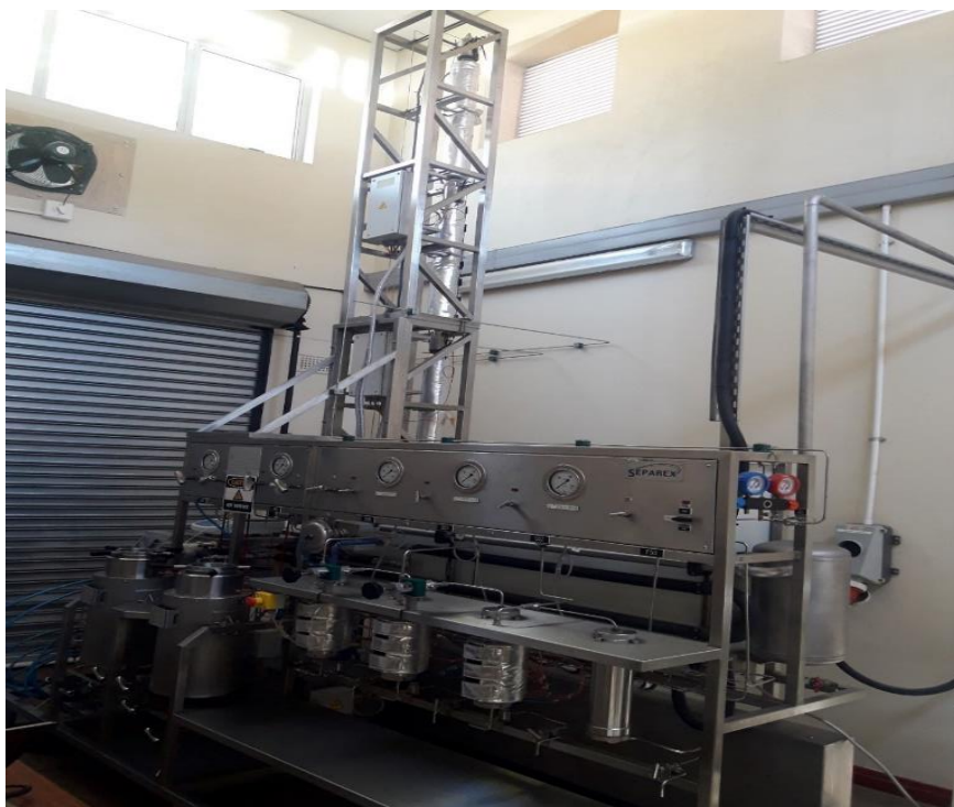
Figure 8.2: Supercritical fluid extraction pilot plant set up for acetoin recovery
