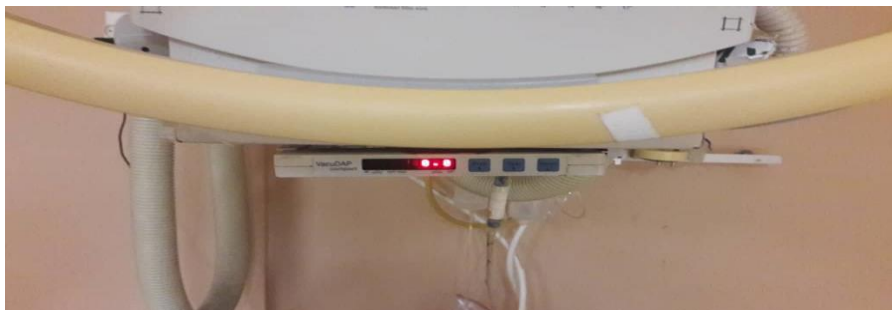
Figure 2.1 KAP meter mounted on the x-ray collimator at one of the research sites.
