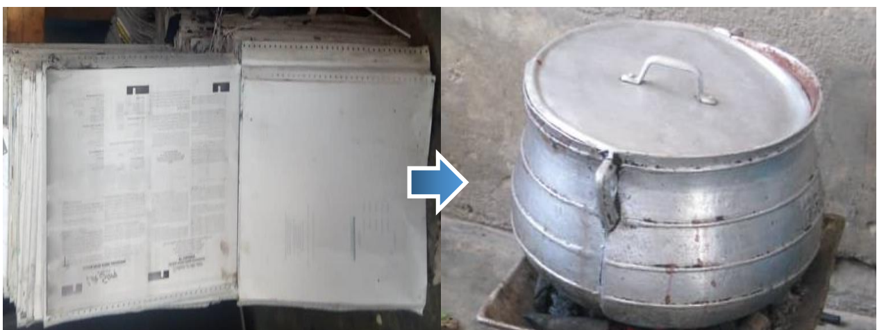
Figure 6.7: Used offset printing plates converted into a cooking pot (Author's photograph 2019)
