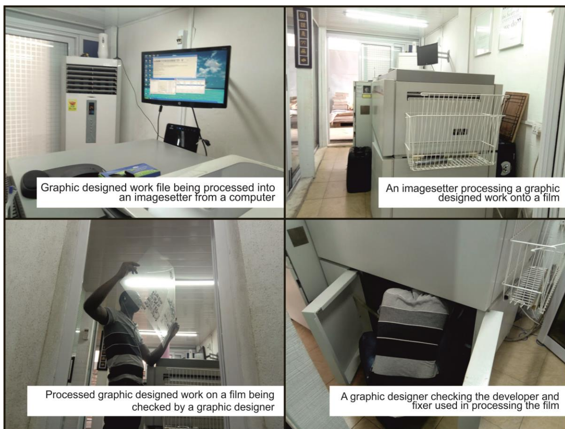
Figure 5.14: Graphic designed work being separated into process colours and processed onto films with an image-setter (Author's photograph, 2019)
