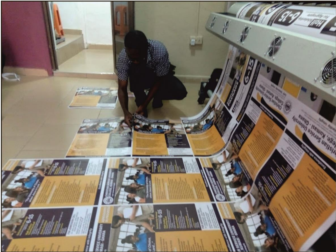
Figure 5.15: Large format digital printer printing design on a self-adhesive vinyl (Author's photograph, 2019)
