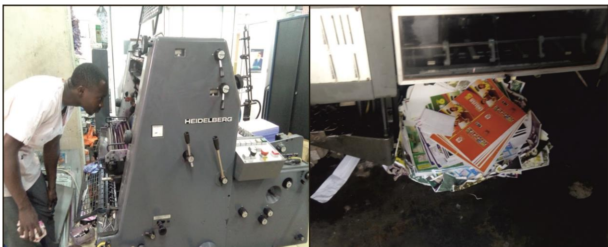
Figure 5.17: An offset printing machine minder about to clean a blanket with printing test sheets next to it (Author's photograph, 2019)
