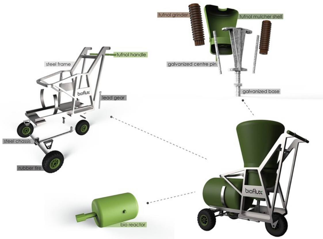
Figure 5.4.7.1: Bioflux exploded view (Bioflux student group, 2019)
