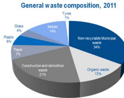
Figure 2-1: The waste composition for general waste, 2011 (percentage by mass) (Department of Environmental Affairs and Tourism, 2012)
