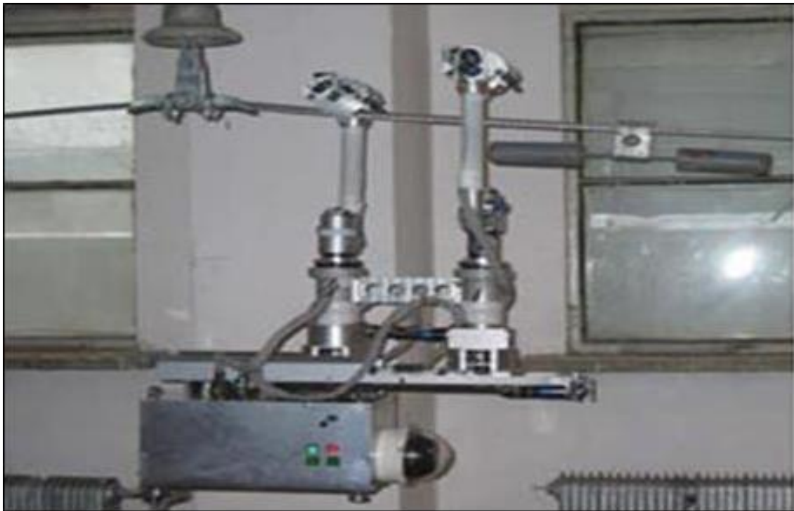
Figure 2-36: The CAS robot crossing a vibration dampener (Zhu, et al., 2006).
