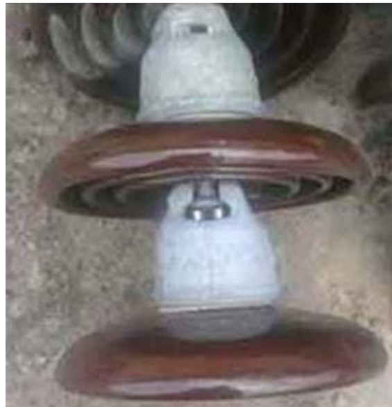
Figure 2-5: The porcelain insulator. (Lancaster, 2012)
