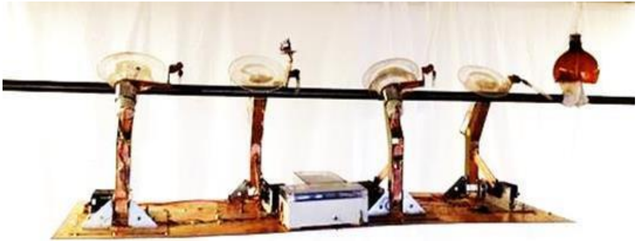
Figure 5-17: The robot approaches an obstacle on the line.
