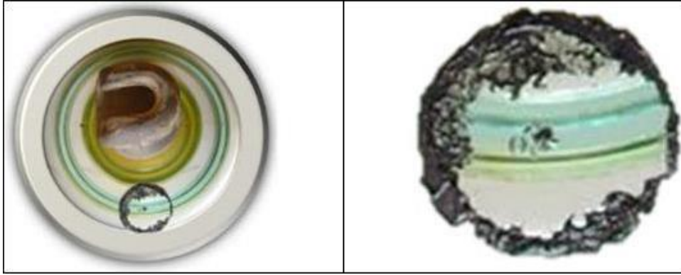
Figure 5-11: Cleaning starts from the centre of the contaminated area, 90 seconds run time.
