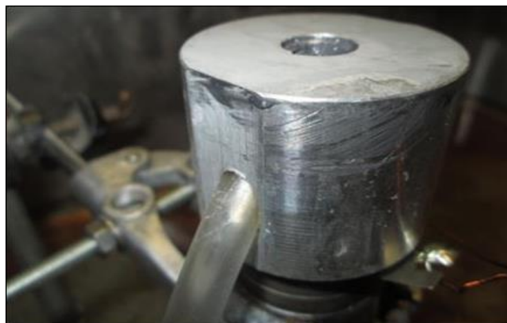
Figure 4-3: The hole drilled through the transducer.
