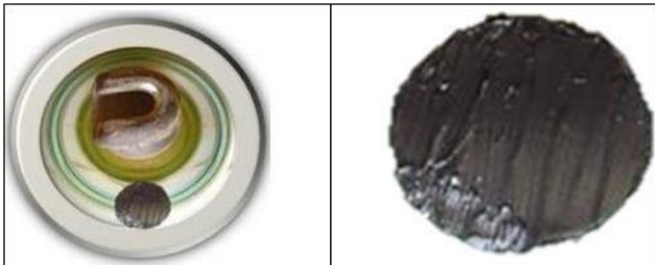
Figure 5-9: The 1 mm layer of grease applied to the surface of the insulator.
