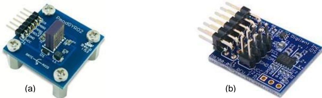
Figure 2-49: (a) Gyroscope and (b) Accelerometer sensor (Mantech Electronics, 2015).
