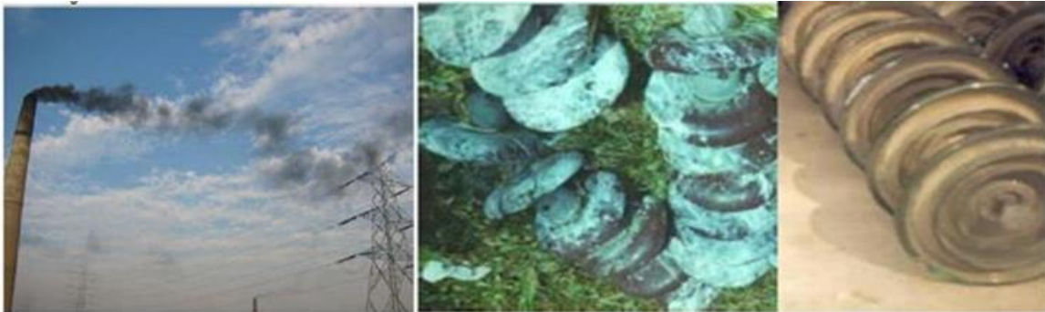
Figure 2-8: Contaminated insulators due to industrial pollution (Kumar & Kumar, 2012).
