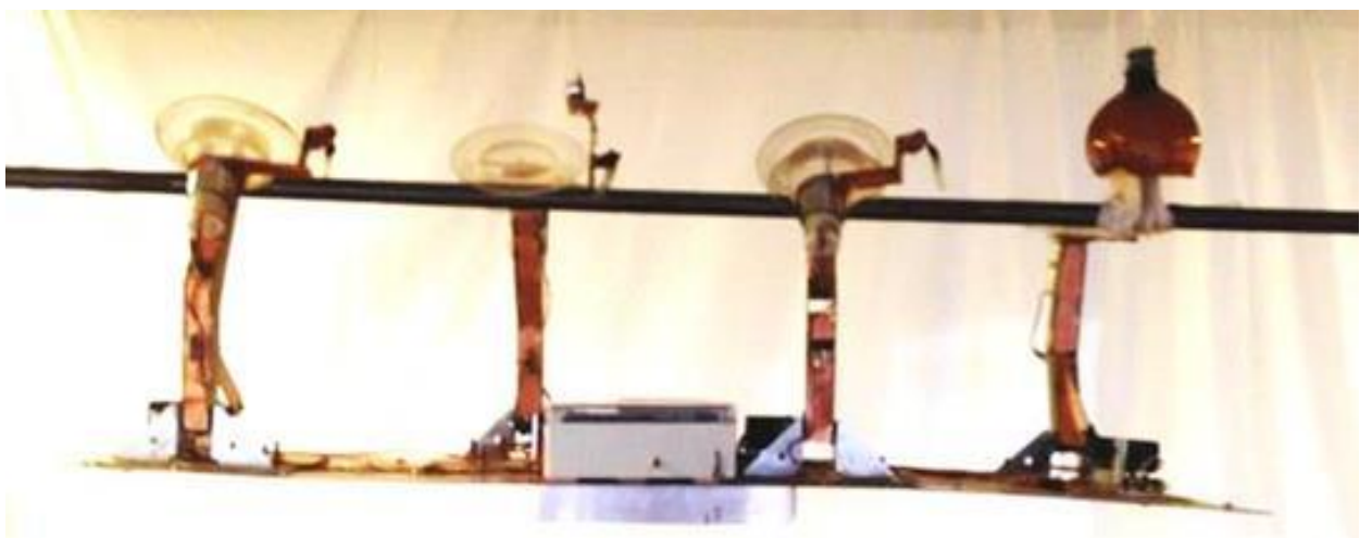
Figure 5-18: The first wheel is removed from the line.
