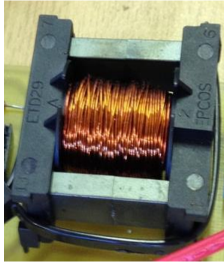
Figure 4-8: The transformer windings wrapped around the ETD29 core.
