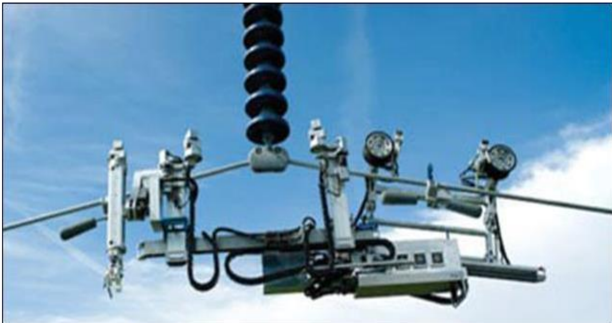
Figure 2-35: The LineScout crossing an insulator string (Pouliot & Montambault, 2009).
