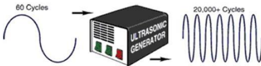
Figure 2-24: Signal transformation after the generator (Fuchs, 1995).
