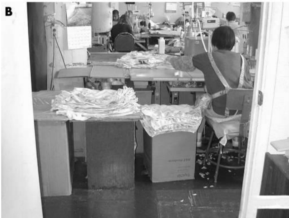
Figure 2.2 Typical machinist stations; (A) operator leaning forward, (B) operator using non-adjustable chair and boxes to support incoming fabric.
