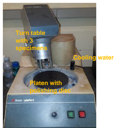
Figure 3.8: Struers LaboPol 5 polishing machine
