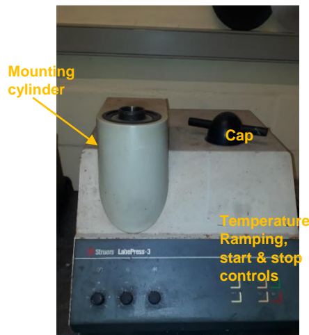
Figure 3.7: Struers LaboPress-3 hot mounting press
