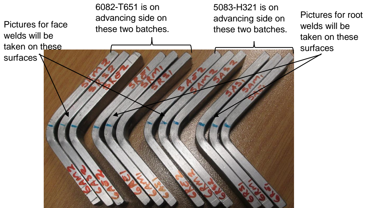
Figure 4.12: Bent dissimilar welded joints
