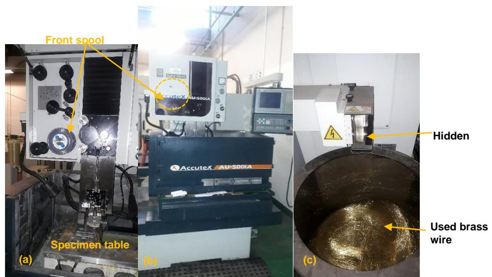
Figure 3.6: (a) Inside spool and specimen table, (b) EDM Accutex AU-500iA wire-cut and (c) hidden spool and brass wire
