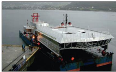
Figure 1.2: Hull structure made of AA5083 Marine Aluminium [Kumar et al., 2015]
