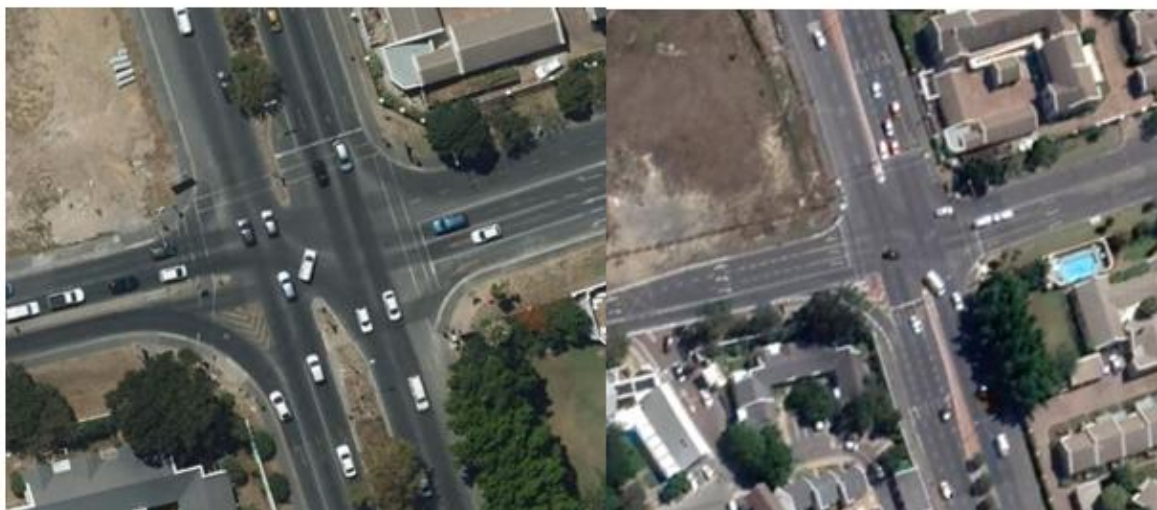
Figure 3.3 Andries Pretorius intersection: left-before upgrade and right-post upgrade (Google Maps)
