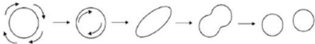
Figure 2:2: Droplet breakup during emulsification (Akbari & Nour, 2018)
