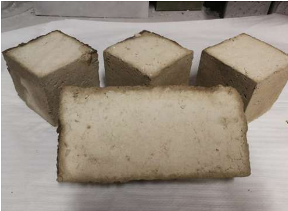
Figure 4.6-1: Light weight geopolymeric bricks produced from South African Lethabo classified coal fly ash.
