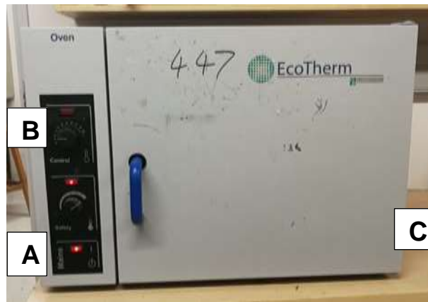
Figure 3.4-1: EcoTherm drying oven: (A) main switch I, (B) control, (C) door.
