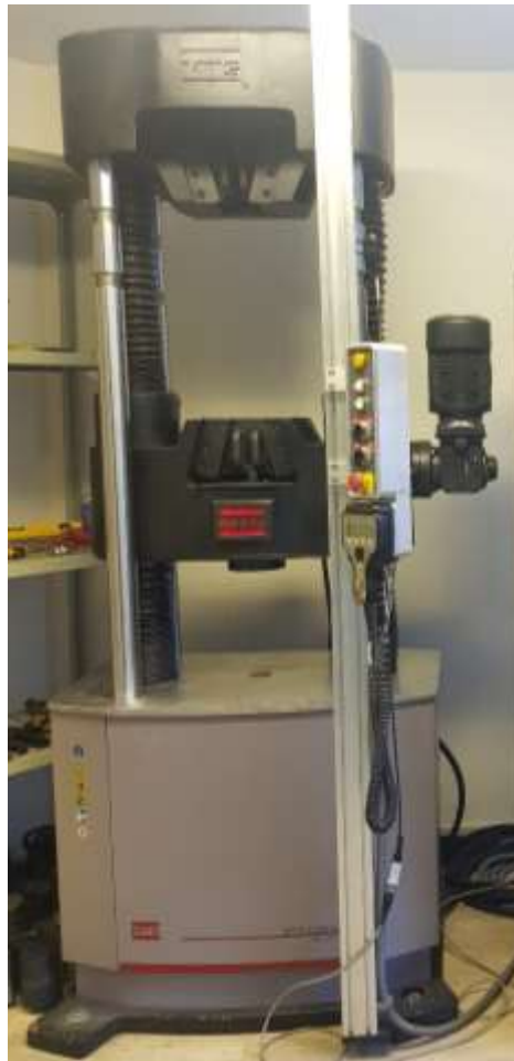
Figure 3.8-1: Compressive strength test machine.
