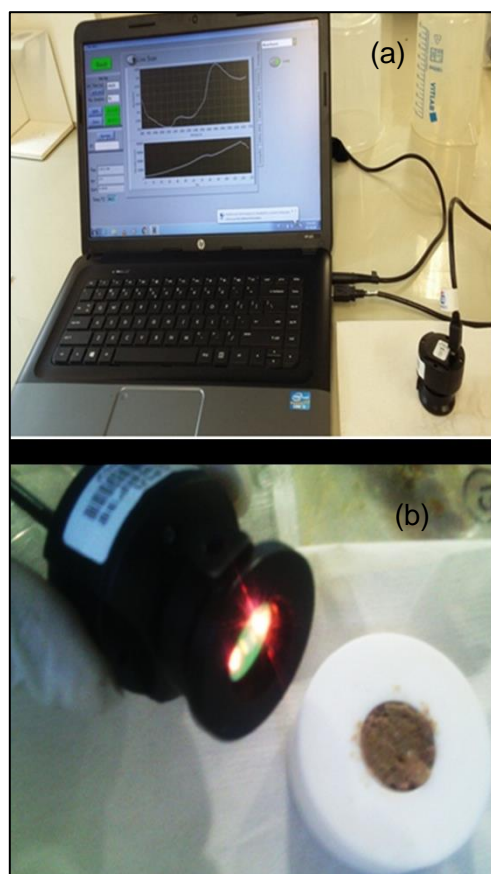
Figure 3.4: (a) Photo illustration the MicroNIR instrument connected to a laptop and (b) a MicroNIR next to a hollowed-out Teflon disk with a homogenised fish sample inside as it was used during the scanning of individual homogenised fish samples. Photos were taken using a Huawei P30 Lite.
