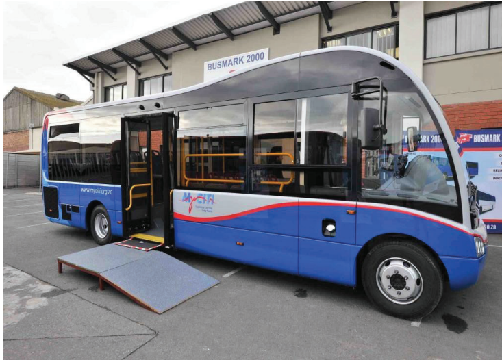
Figure E.8: Universal access system on MyCiTi bus (Source: Our Future Cities, 2019)
