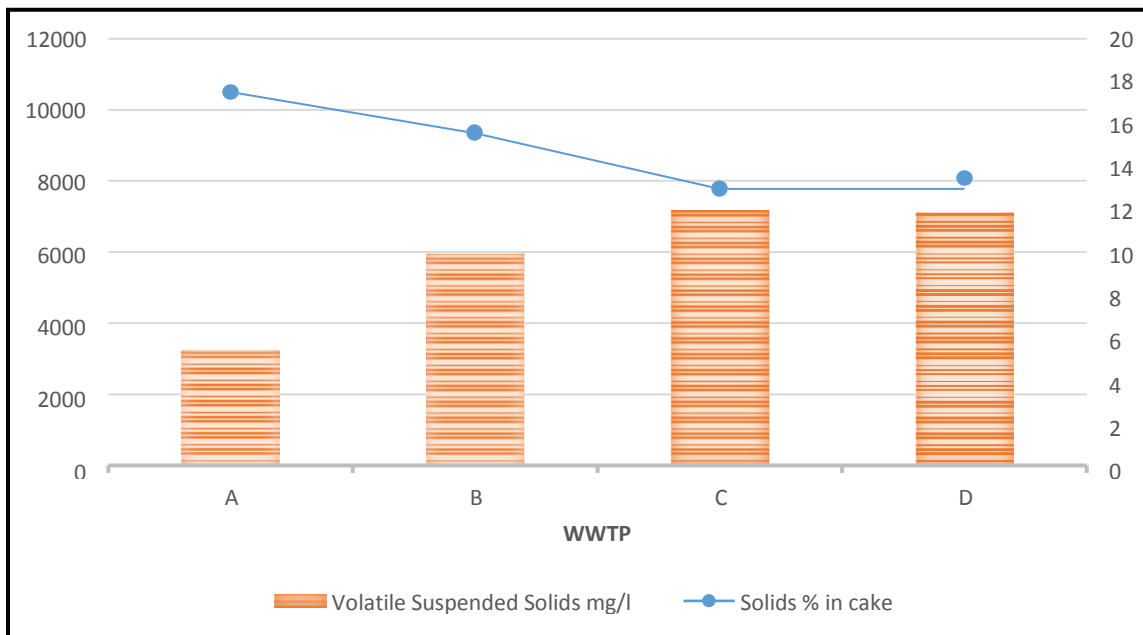
Figure 4.1: Volatile suspended solids effects on cake dryness
