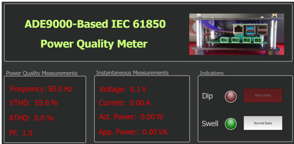
Figure 8-18: The SCADA HMI with MMS Client Connected and GOOSE Publishing Enabled but no Current or Voltage Injected
