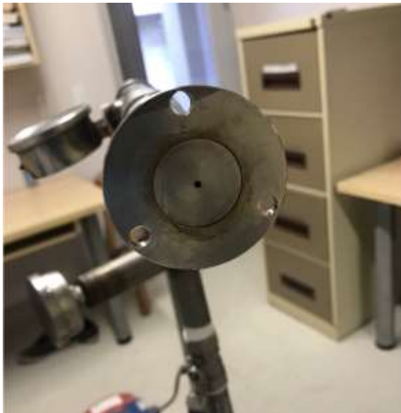
Figure 0-3: An orifice plate and its slot in the HC Jet loop system
