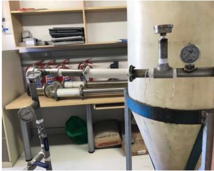
Figure 0-4: A part of the HC Jet loop system containing the venturi
