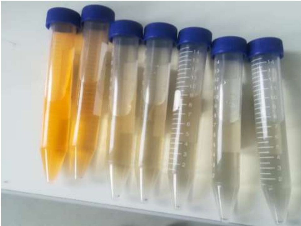
Figure 0-5: From left to right 0 min: 10 min samples collected when decolourising 10 L of 20 ppm OR2 in the HC jet loop system for 10 min using a 2 mm hole diameter orifice plate and 400 kPa inlet pressure
