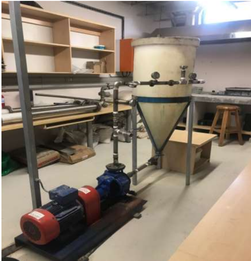
Figure 0-2: Set-up of the HC Jet loop system
