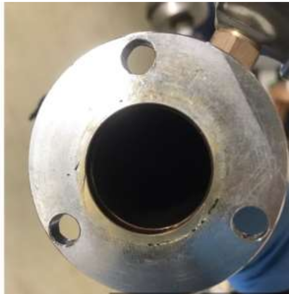
Figure 0-3: An orifice plate and its slot in the HC Jet loop system
