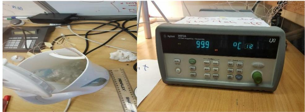
**Figure 3.28: Thermocouples Inserted in boiling water in the kettle**
