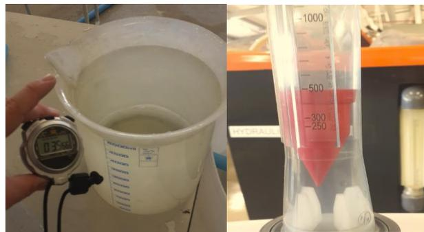
**Figure 3.33: Flow rate measurement using beaker, stop watch and variable area flow meter**
