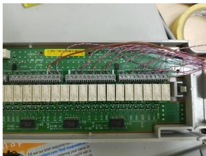
**Figure 3.27: Agilent data logger circuit board (24 channel multiplexer)**
