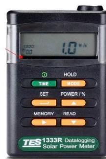
**Figure 3.35: Solar radiation meter**
