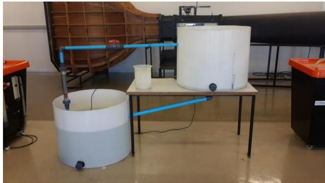
**Figure 3.32: Flow rate test calibration set-up**
