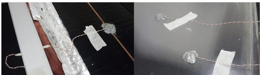
**Figure 3.25: Thermocouple set-up**
