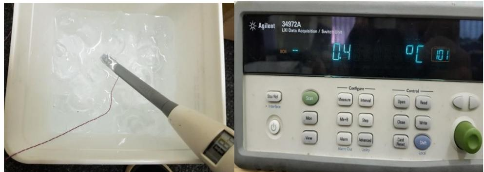
**Figure 3.29: Thermocouple's calibration in water and ice mixture in a bucket**
