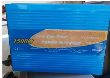
**Figure 3.14: KS-1500P 1500 W 24 V inverter**
