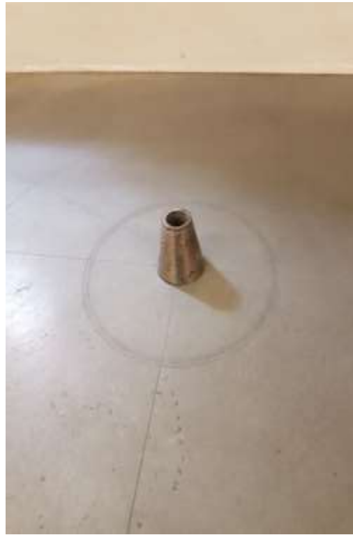
Figure 3.5: Mini-slump cone on top of baseplate before pouring the sample
