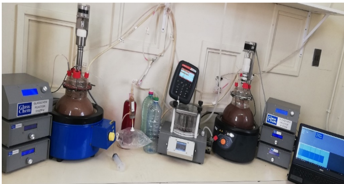
Figure 3-8: Photographic image of the 5L laboratory-scale experimental AD set-up
