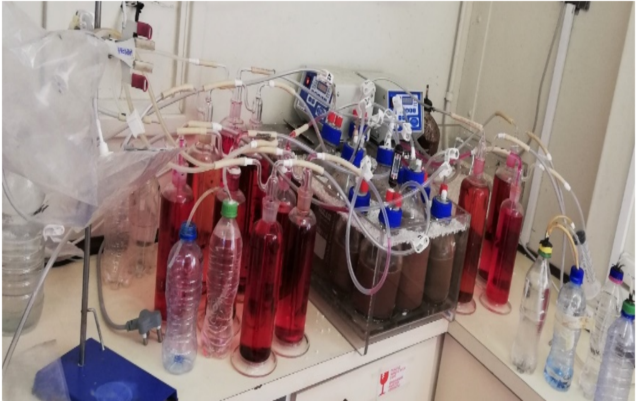
Figure 3-6: Photographic image of BMP assay experimental set-up
