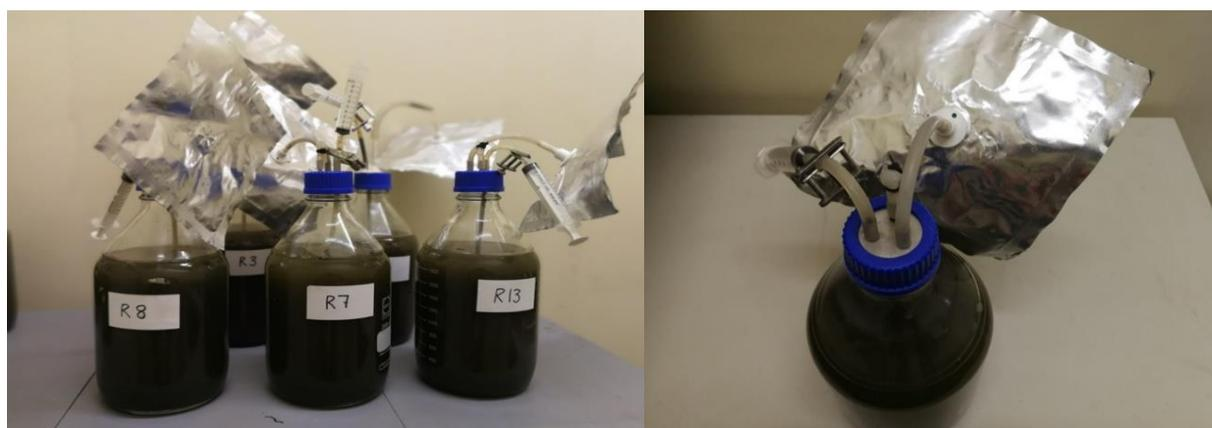
**Figure 3.2: Biochemical methane potential test set-up**
