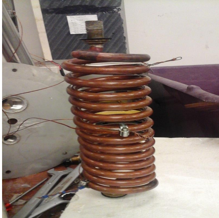
Figure 3.6: Heat exchanger helical coiled copper pipe
