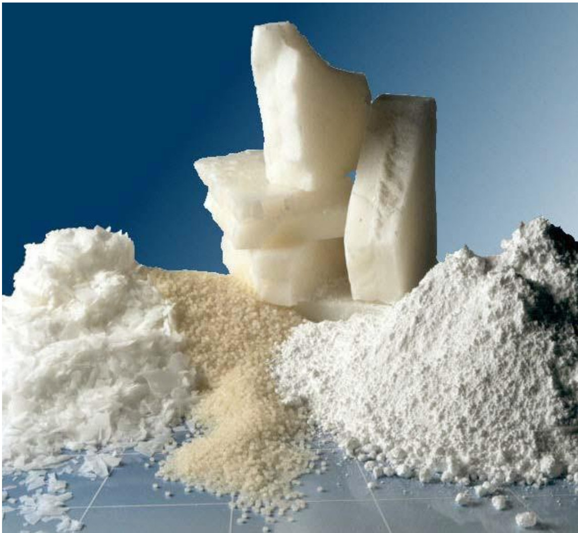
Figure 0.1: Phase change materials based on n-paraffins and waxes (Rubertherm, 2019)
