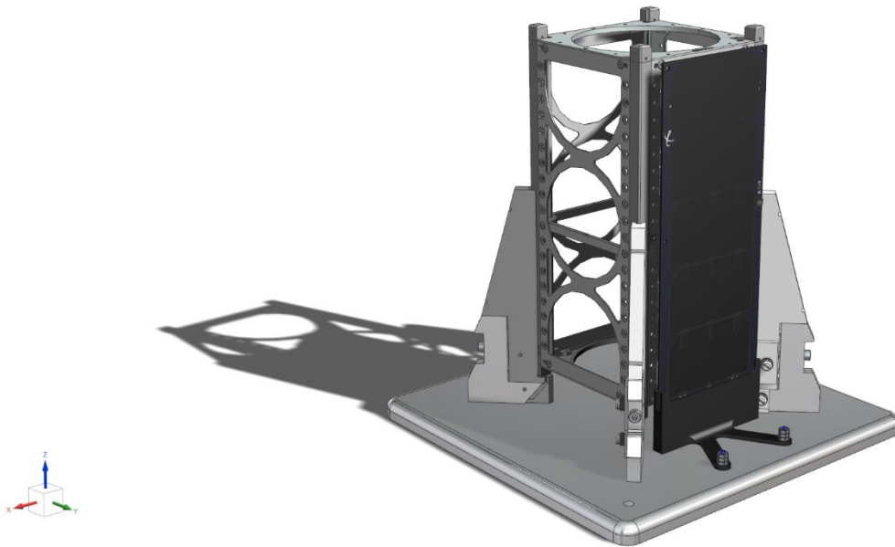
Figure 6-89: Solar panel mount in position
