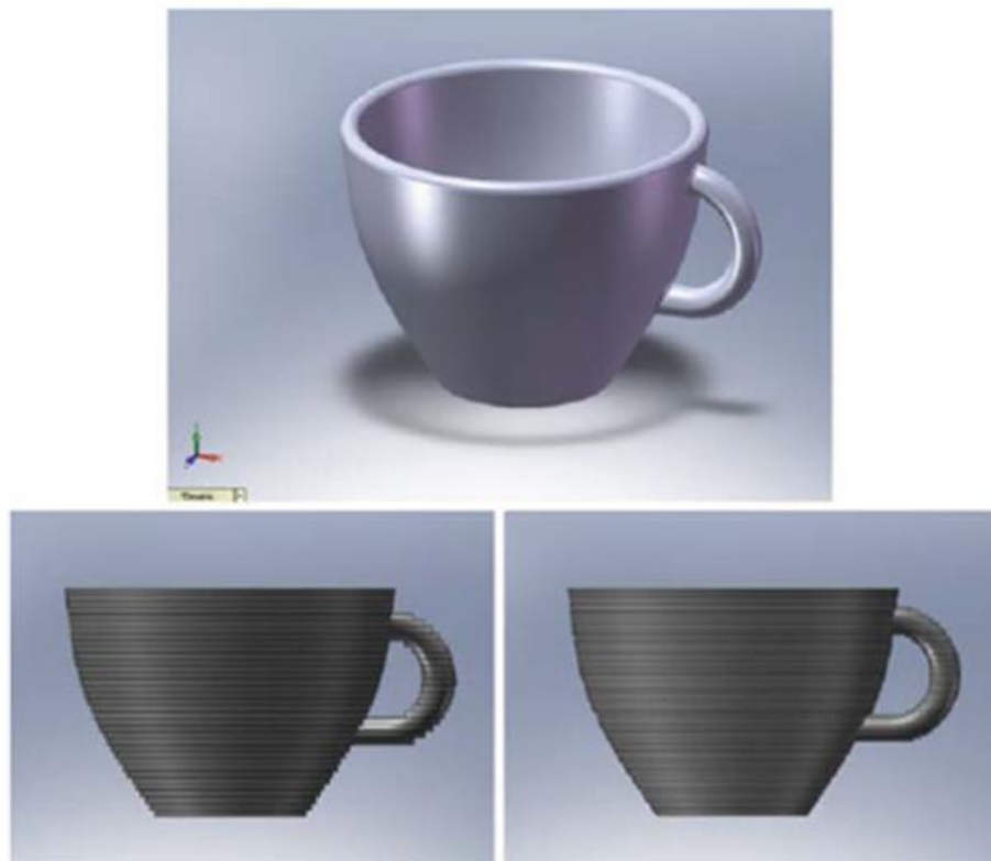
Figure 1-10: Thin vs thick layer build (Gibson et al., 2015)
