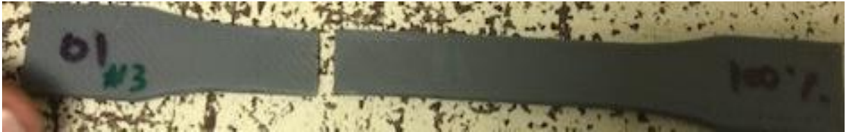
Figure 6-82: Three broken 100% PLA tensile test specimens
