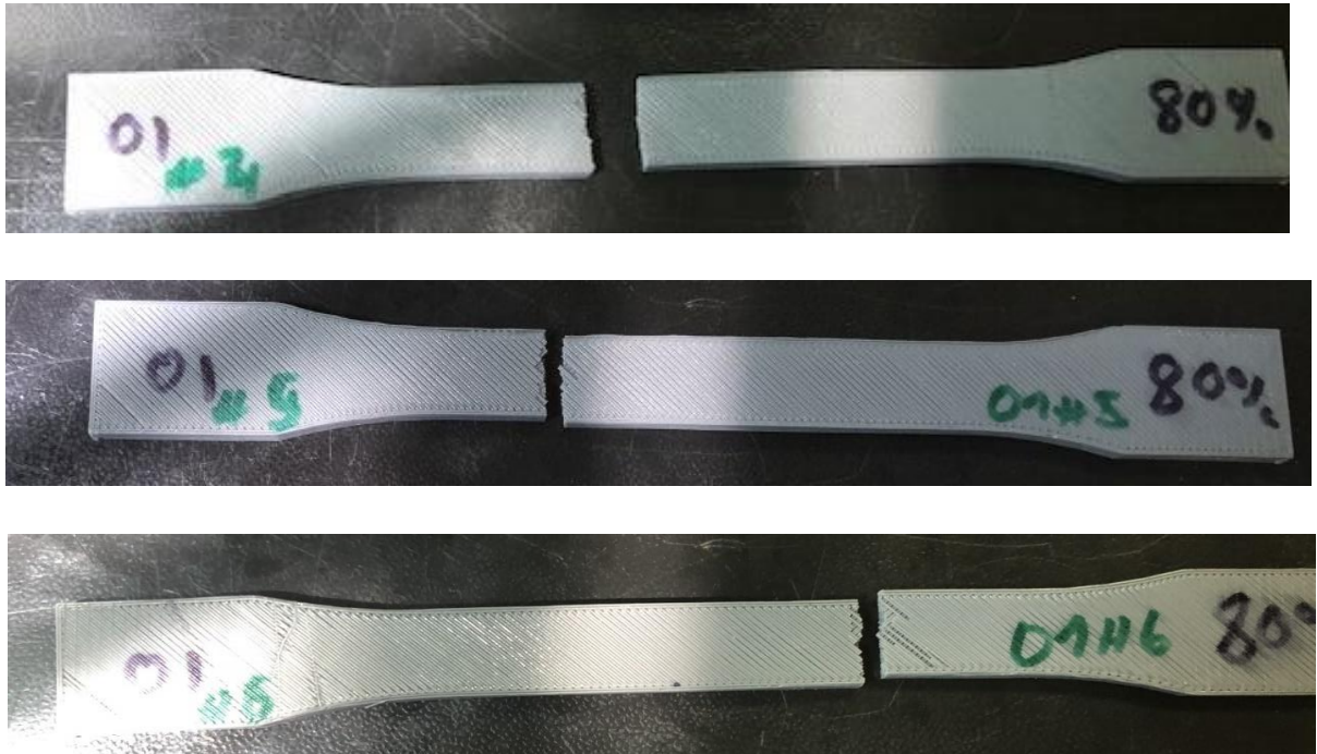
Figure 6-81: Three broken 80% PLA tensile test specimens
