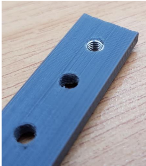
Figure 6-5: Helical insert in the tapped hole
