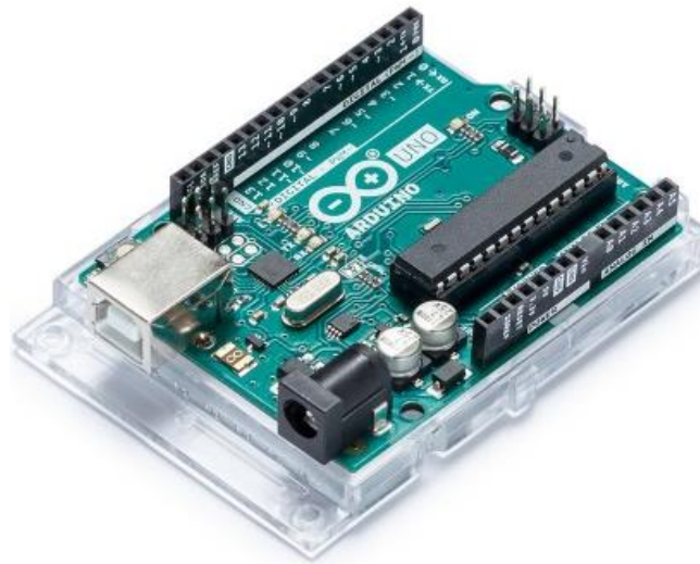
Figure 38: Arduino Uno ATmega328PU programming board.
