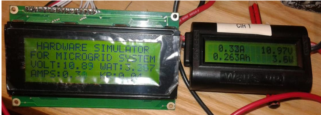
Figure 40: LCD Display calibration
