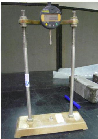
Figure 2.5 Comparator – to measure change in length of concrete specimen (Tam, Tam & Ng, 2012).
