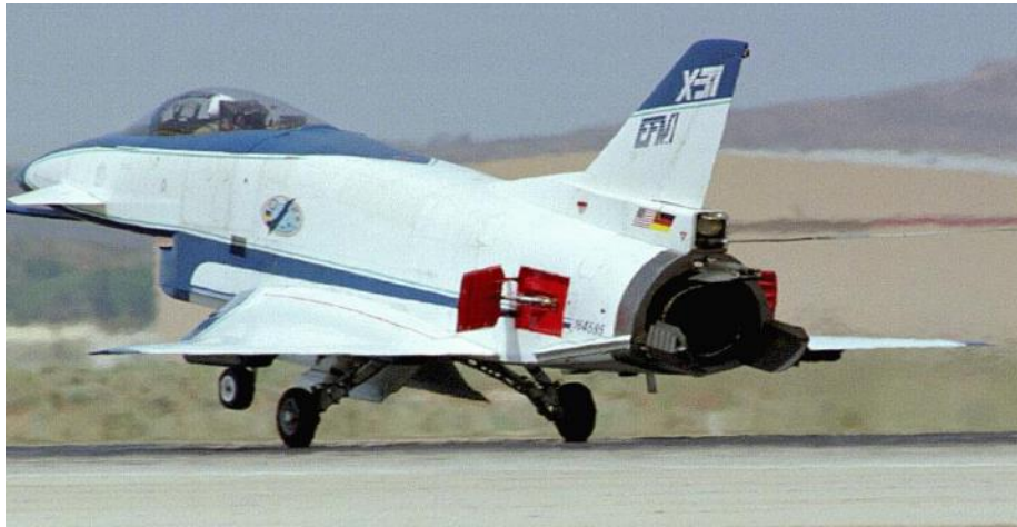
Figure 2.1: X-31 with canard fore planes (Rockwell-MBBX-31, 1990)
