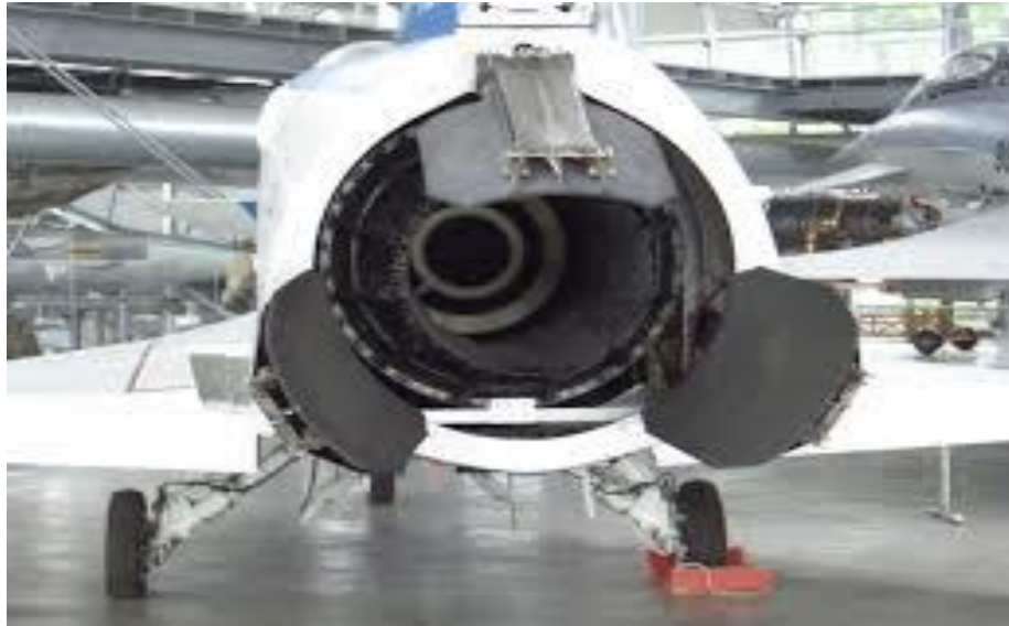
Figure 2.15: Vane thrust vectoring system (Clarke, 2011)
