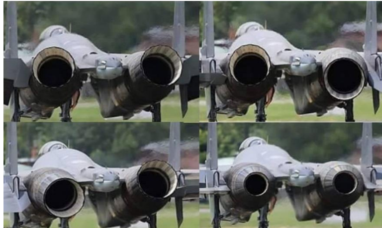
Figure 2.20: Gimbaled thrust vectoring system for jet engine aircraft (AviationNepal, 2017)
