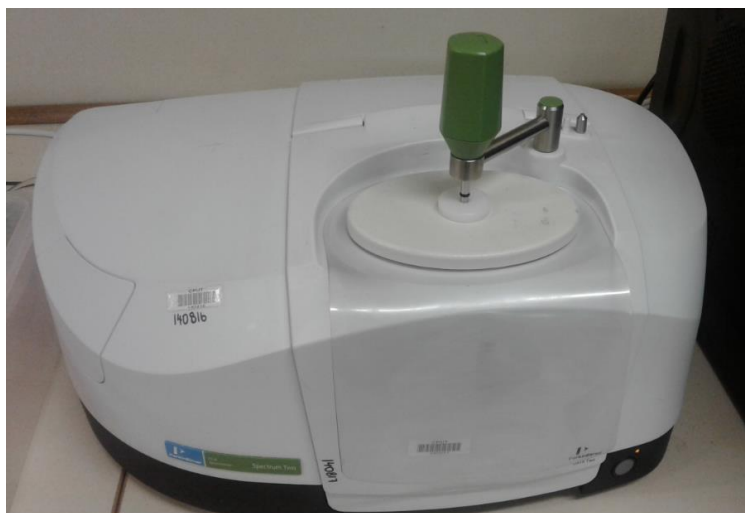
Figure: 0.3: Perkin Elmer universal total reflectance Fourier Transform Infra-Red spectrum II spectrometer
