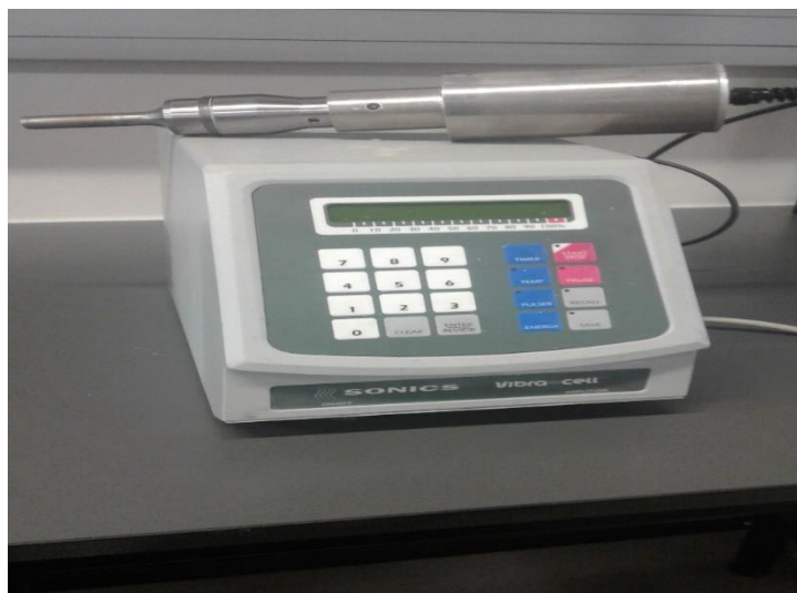
Figure: 0.5: Ultrasonic processor used in the formulation of O/W-type nanoemulsions
