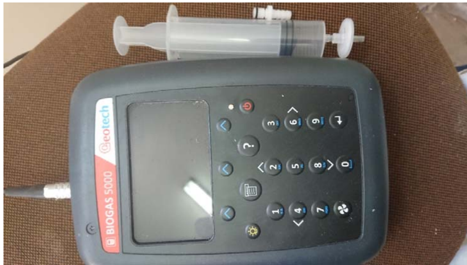
Figure 3.6: Biogas 5000 Geotech Analyser
