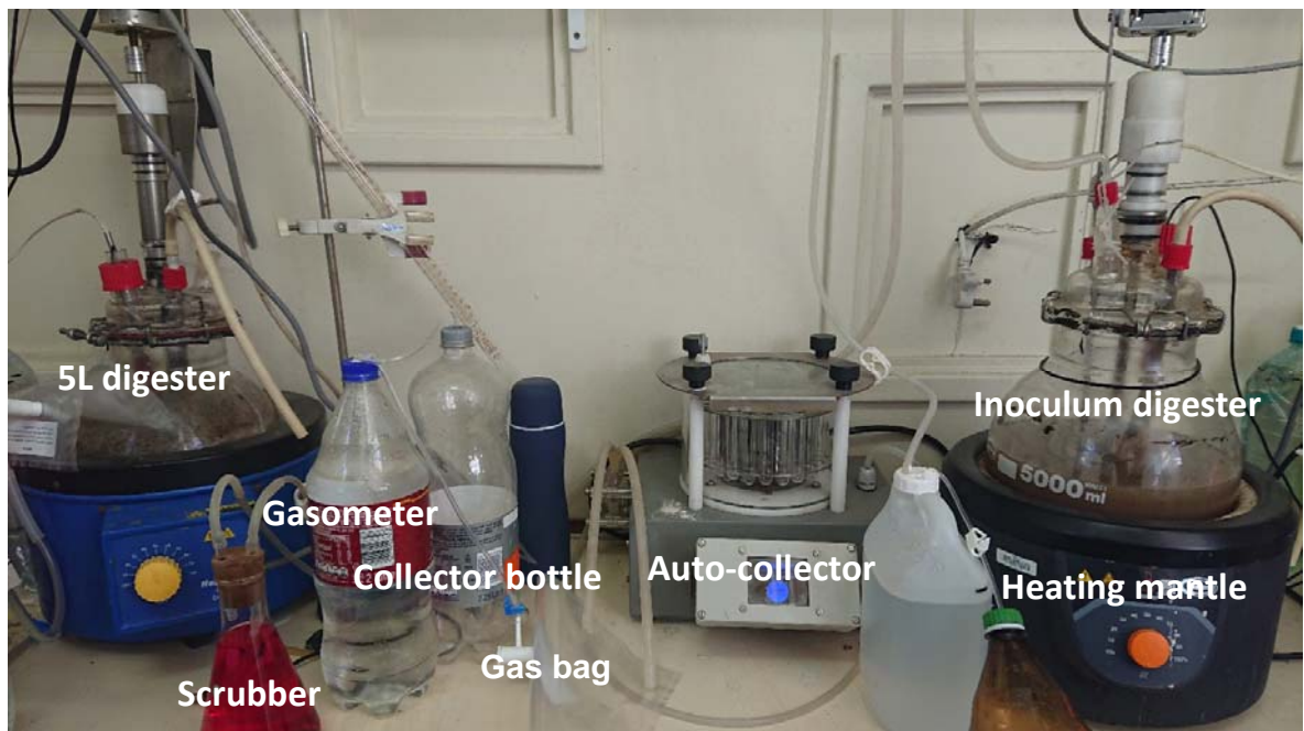
Figure 3.7: 5L single stage mesophilic digester set-up for upscaling
