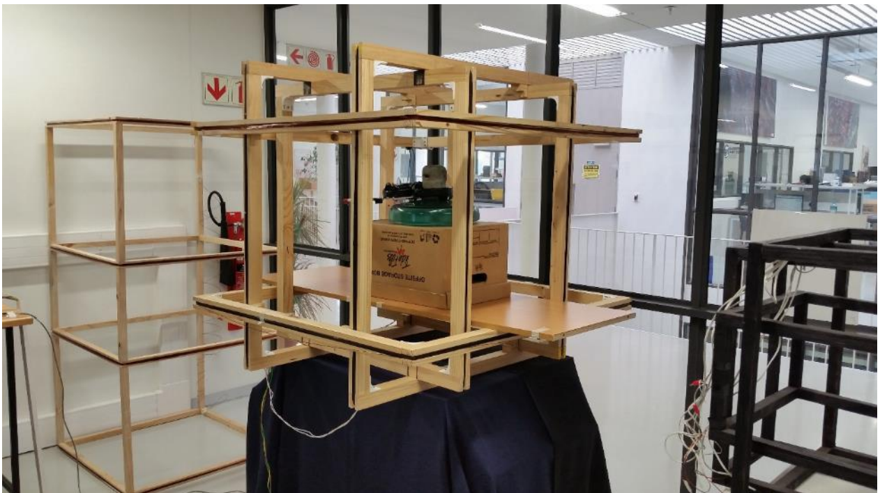
Figure 4.31: LCPR2 sensor placed around an insulator inside the Helmholtz coil at CPUT
