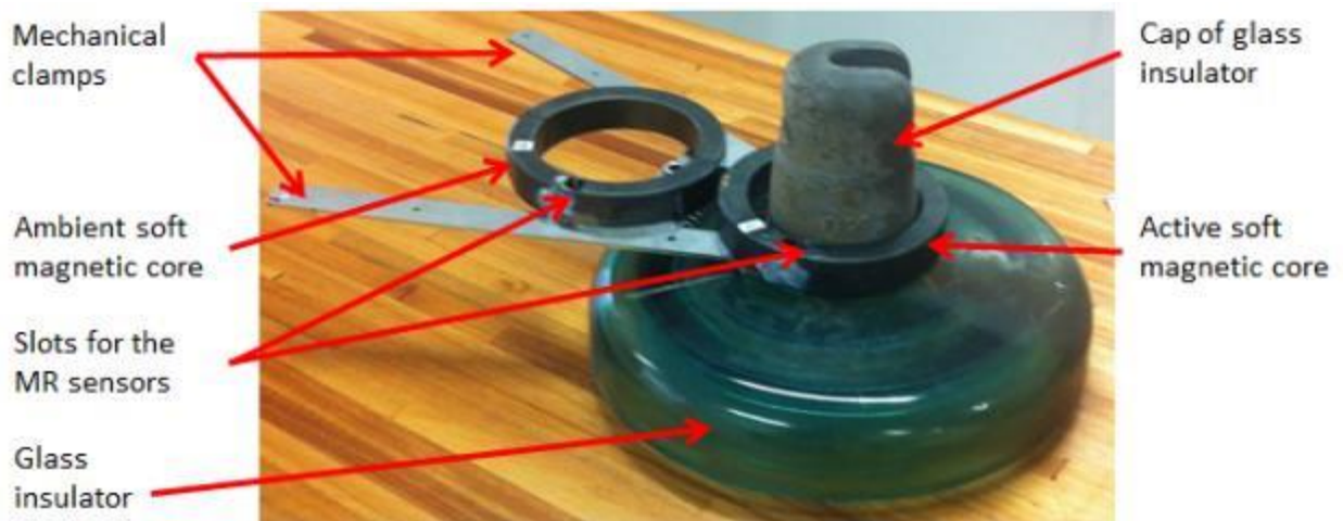
Figure 4.27: LCPR2 sensor with its mechanical clamps around a glass insulator
