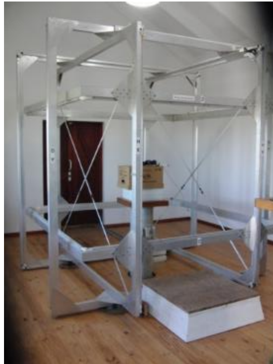
Figure 4.36: LCPR2 sensor placed within the working volume of the SANSA's Helmholtz coil
