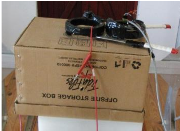
Figure 4.37: Current carrying wire passed through the LCPR2 for linearity tests
