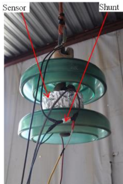
Figure 5.3: Position of the LCPR1 sensor and shunt resistor in the calibration setup of Figure 5.2
