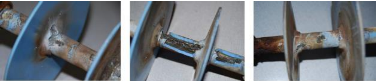
Figure 2.7: Comparison of material aging of an HTV SR insulator under HVAC, positive HVDC and negative HVDC excitation, respectively (From Limbo, 2009)
