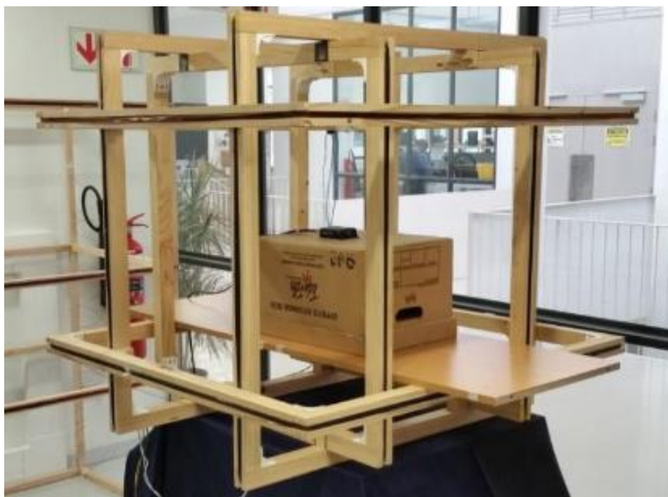
Figure 4.29: LEMI-011B fluxgate magnetometer inside Helmholtz coil at CPUT
