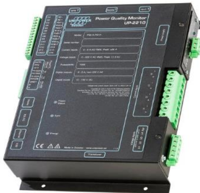
Figure 6.36: Unipower 2210 Class A measuring unit Adapted from Unipower (2013)
