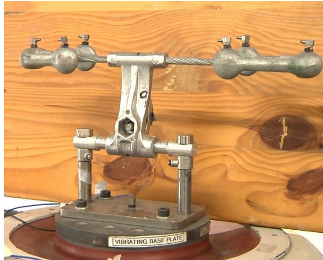
Figure 5. 15: The asymmetric Stockbridge damper with two accelerometers on the inner part of each mass.
