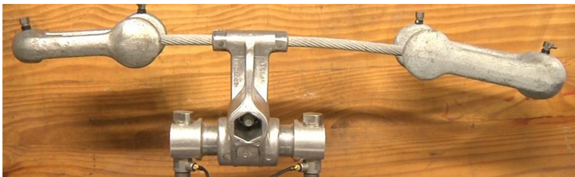
Figure 2. 6: Claren and Diana damper with four accelerometers (4-R Stockbridge-type Damper)
