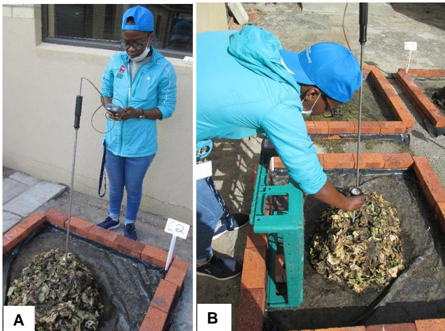
Figure 2.5: Measuring compost heap temperature data (A) and recording pH & moisture content of the compost heaps (B).
