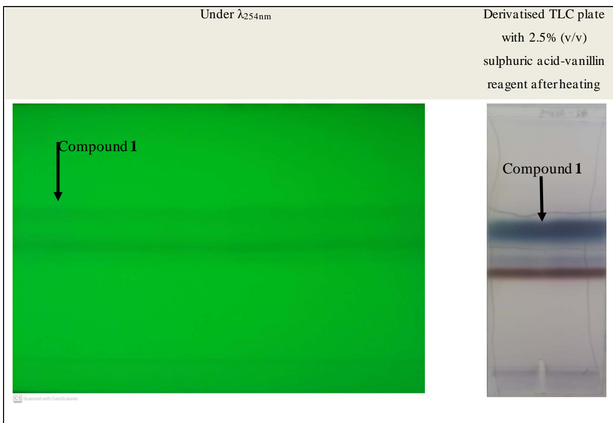
Figure 3-4 Preparative TLC for the isolation of compound 1. Plate developed at 97:3 hexane: ethyl acetate (double run)
