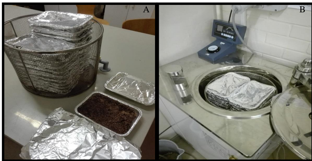
Figure 5.1: Foil containers were half filled with medium and covered with single layer of thick aluminum foil (A) and then autoclaved at 121°C for 15 minutes twice (B).
