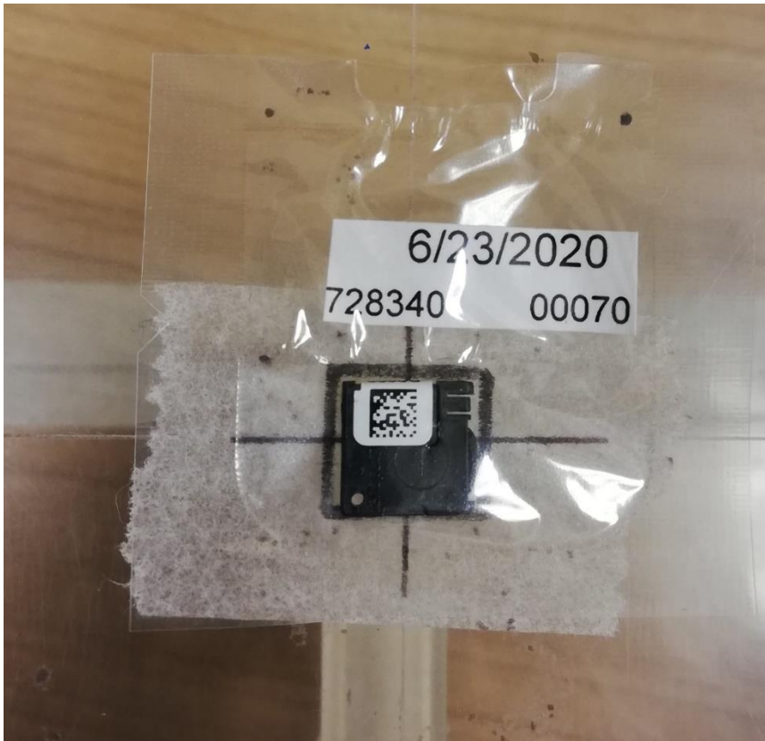
Figure 3.49: The square enabled quick positioning of the nanoDot dosimeters (Photo taken by the researcher)
