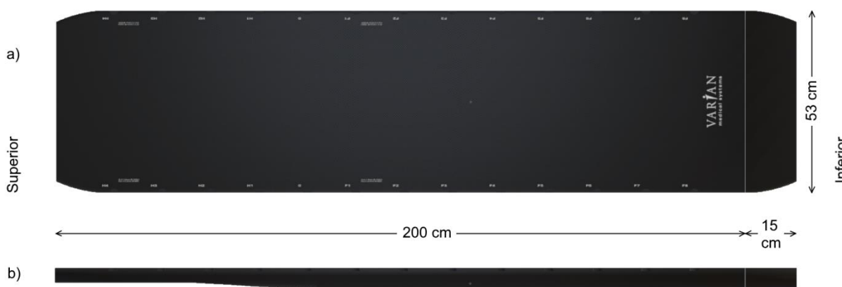
Figure 3.1: The main dimensions of the Varian IGRT couch
