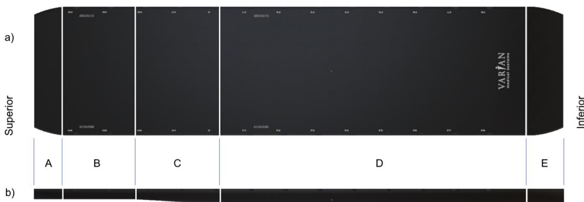
Figure 3.3: Indicating the five (5) main sections of the Varian IGRT couch
