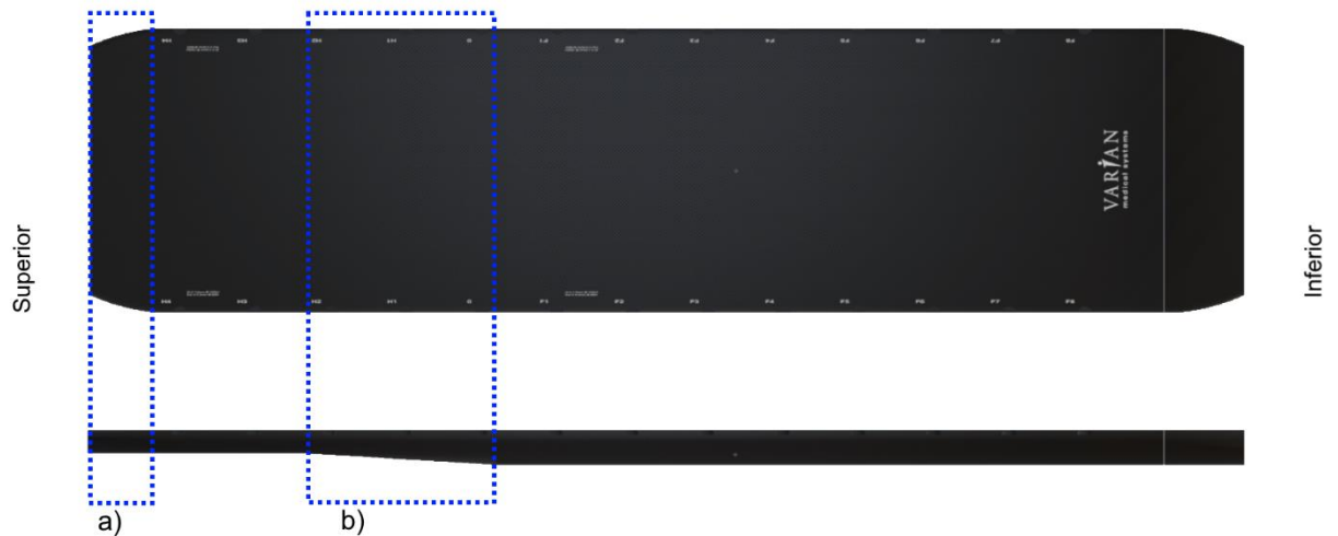
Figure 3.28: The two regions of the couch where interpolations were required to create the external shape of the couch, the superior region (a) and the sloping section (b)
