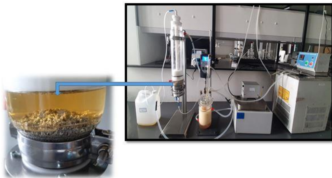
Figure 3.6: Continuous transesterification set-up used in this study
