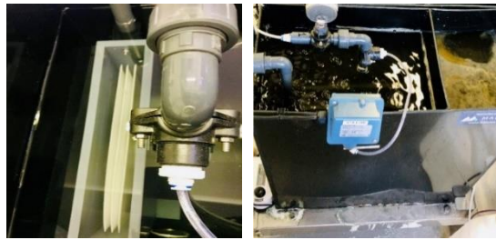
Figure S5: Photographic illustration of the submerged ultrafiltration membrane (left), and membrane tank (right).
