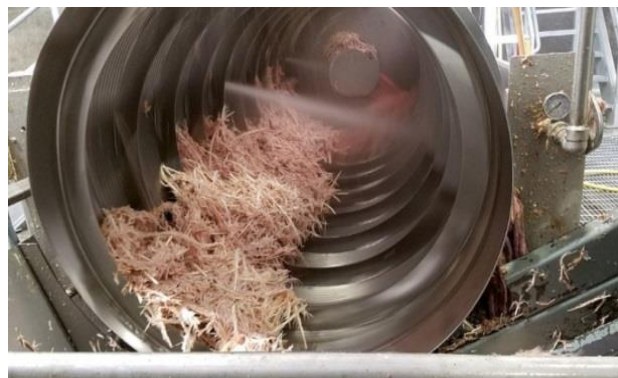
Figure 2.3: Rotary cylindrical screen used at a poultry slaughterhouse in Virginia, United States of America (USA) (Burrows and Reidy, 2018).
