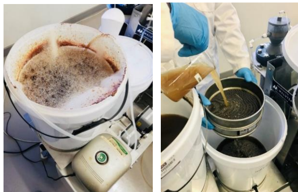
Figure S2: The pre-treatment process in which 20ml Ecoflush™ was added to 20L PSW, aerated for 24h, then allowed to settle for a further 24h before screening and placing it into the 25L feeding tank.
