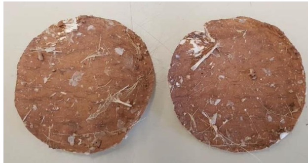
Figure 4.1: Image showing the residue of PSW on the 1.0µm glass fibre filter after filtration.
