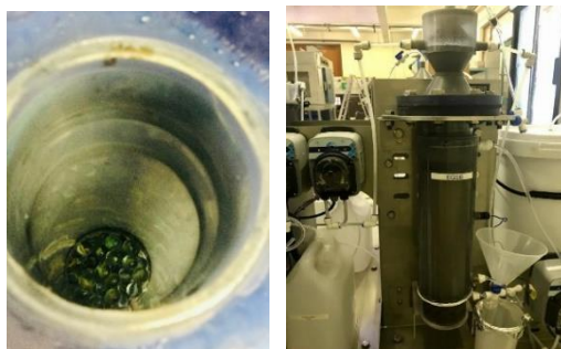
Figure S3: Photographic illustration of the glass marbles underdrain system and the EGSB reactor.
