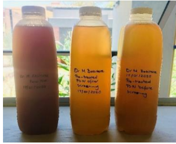
Figure 5.8: Bottles containing raw PSW (left), pre-treated PSW after screening (middle) and pre-treated PSW before screening (right).
