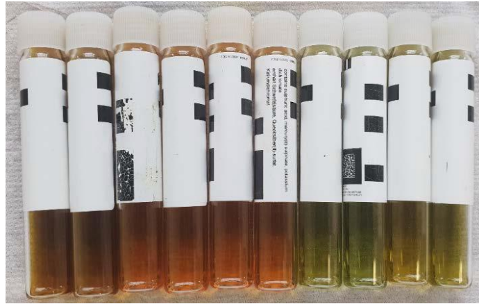
Figure 4.2: COD fractions (total, filtered and flocculated filtered COD) in analysis test tubes.
