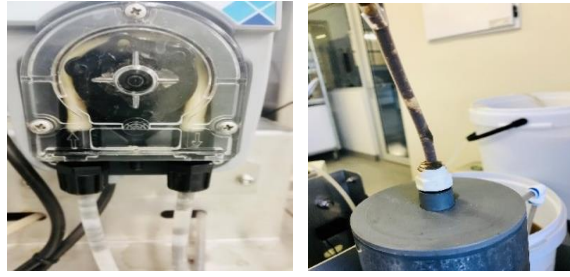
Figure S4: Sludge washout in the EGSB recirculation stream (left), and biogas gas line (right).
